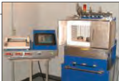
FIGURE 3. The Schulze Ring Shear Tester (RST) provides the benefits of the fully automated, full scale RST in a compact package. This tester for fine chemical applications requires only 3.5 mL of sample
