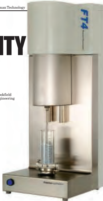
FIGURE 2. The Freeman Technology FT4 Powder Rheometer, a universal powder tester, offers three instruments in one. It combines a patented blade methodology for measuring flow energy with a range of shear cells, wall friction modules and other accessories for measuring bulk properties
